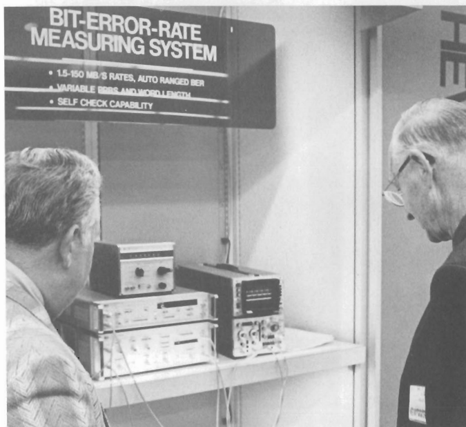
Developed and manufactured at the South Queensferry, Scotland facility, the new HP bit-error-rate measuring system is designed for use by communications companies to determine the capacity of lines in carrying digital and voice signals as well as to point to trouble in the line. At left in picture is Rudy Poucher, Sacramento district manager for Neely Sales Region.
