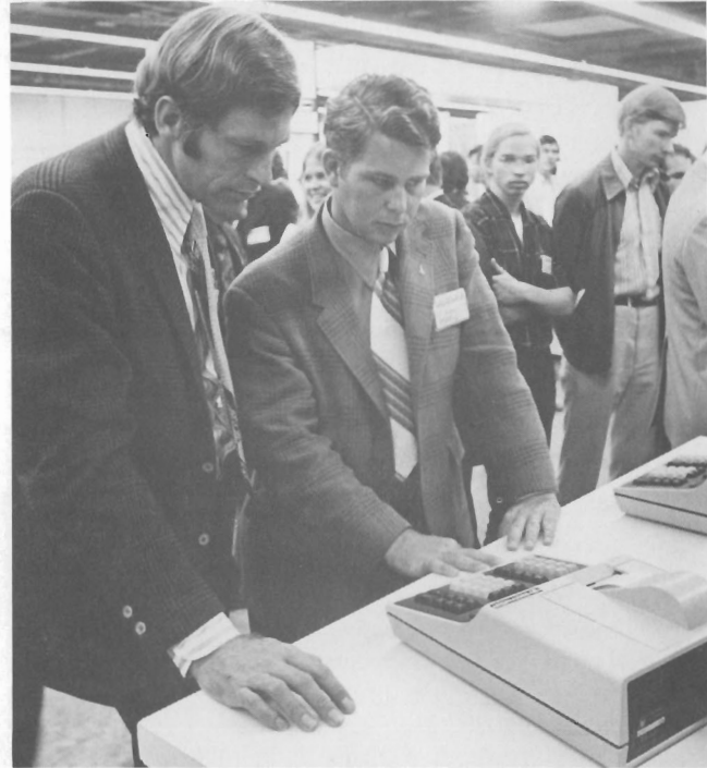
The powerful HP-46 is the desktop version of the HP-45 pocket calculator. Both provide advanced scientific and engineering capability, but the 46 adds a built-in paper tape printer for permanent record keeping. Ed Heinsen, left, Advanced Products Division engineer, demonstrated the 46 and other machines for Wescon visitors.
