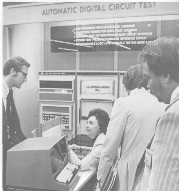
AMD's new 9560B/D digital circuit test system tests printed circuit boards by means of a stored test program rather than by comparison with a reference board. The system can test digital assemblies or boards with up to 360 pins at rates to 22,000 patterns a second.
